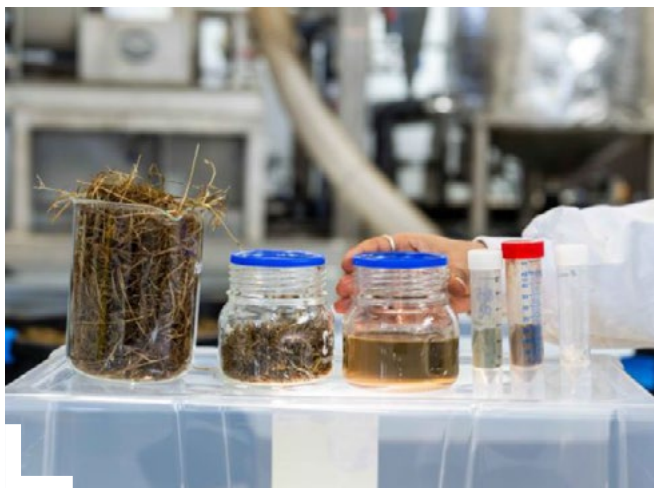
Products made from a small scale grass biorefinery at MTU, these are; silage, press cake and filtered silage juice.
